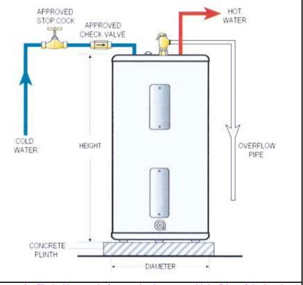
**REMINDER:** Water heater tank must be filled with water before turning it on to avoid dry firing of the heating element
