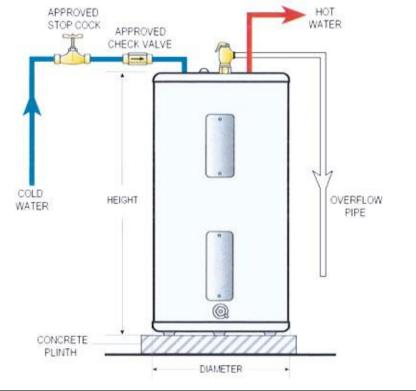
**REMINDER:** Water heater tank must be filled with water before turning it on to avoid dry firing of the heating
