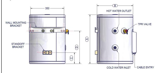
**REMINDER:** Water heater tank must be filled with water before turning it on to avoid dry firing of the heating element.
