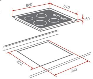
ATTENTION: Cut hole must be with round corners in order to avoid cracking on the counter-top.
