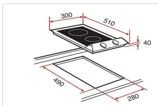
ATTENTION: Cut hole must be with round corners in order to avoid cracking on the counter-top.
