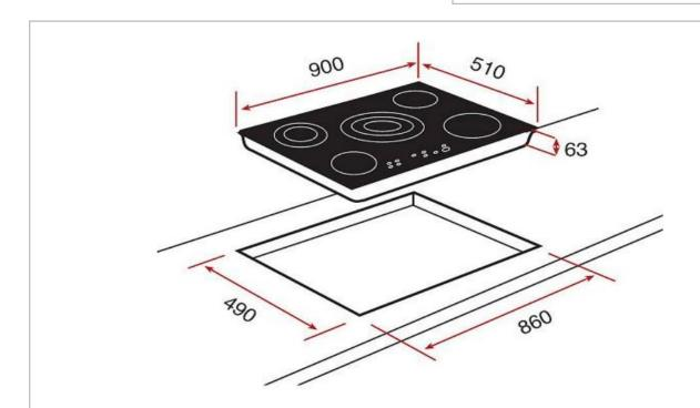
ATTENTION: Cut hole must be with round corners in order to avoid cracking on the counter-top.
