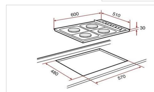
ATTENTION: Cut hole must be with round corners in order to avoid cracking on the counter-top.
