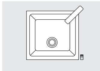
Mixer on the back right, control lever to the right of the sink
