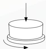
A single, multifunctional control element: 1 push for cold water, 2 pushes for mixed water, 3 pushes for hot water. For individual temperature preference: turn the control. Push and turn to adjust water volume. And the mixer also offers a cleaning mode, temporarily preventing water flow during cleaning and a thermostatic control prevents scalding.
