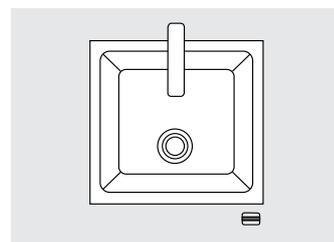
Mixer behind the sink, control element mounted on the front of the kitchen worktop
