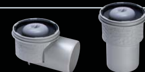
Practicus made of PP, with odour trap, 1.8 l/sec flow rate, sealing water height 50 mm
