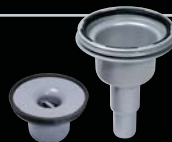
„The Vertical“ made of ABS, vertical outlet Ø 50/40, 1.2 l/sec flow rate, with odour trap for fitting in upper section sealing water height 50 mm 45 254
