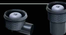
Ecoguss , with odour trap, 1.8 l/sec flow rate, sealing water height 50 mm
