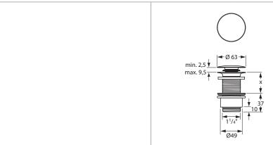
"Flip top" design universal drain valve for basins without overflow
