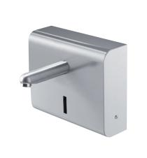
lino exposed wall-mounted faucet K20, with IR-sensor, without temperature-mixing (for cold or pre-mixed water), stainless-steel
