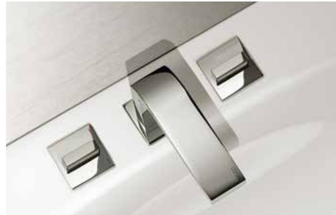
Three-hole fittings with a difference: Temperature regulation on the left, flow rate on the right. After adjusting to your own desired temperature, by pulling it up, the regulator can be returned to its initial position so that the temperature setting is retained.
