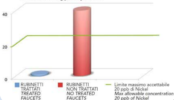
Cessione Nickel da rubinetteria Nickel leaching from faucets
