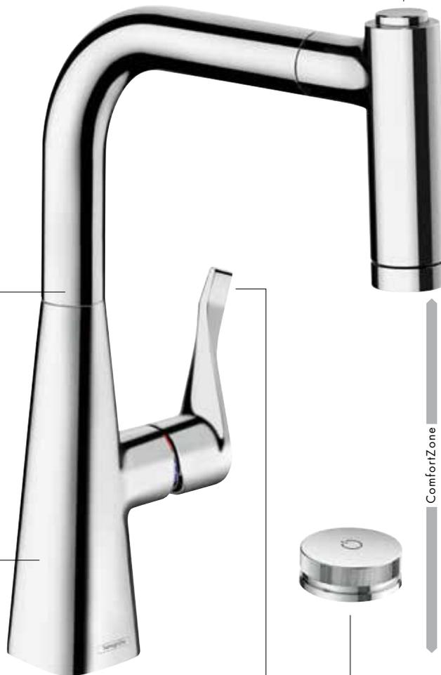
This lever is used to initially start and stop the water, and also to select the water temperature. The water can be stopped or restarted at any time using the Select button on the front edge of the sink while still working.
