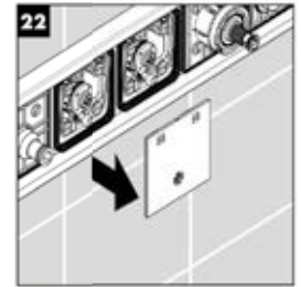
Removing the template
