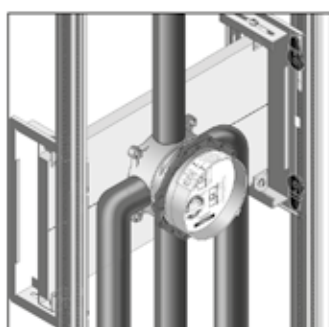
Installation on carrier system
