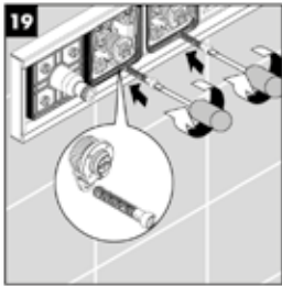
Fitting the adjustment screw for Select valves
